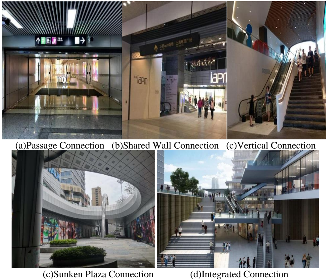
Figure 1: Subway Underground Station Connection Methods with Surrounding Underground Spaces
